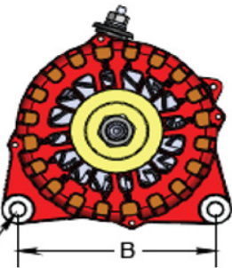
Mounting Foot Bore: VT - 3/8" (10mm)
