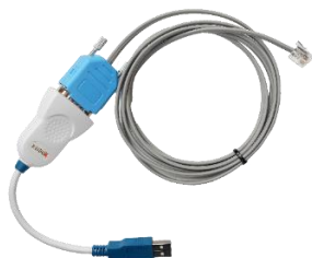
Fig 1: Programming Cable & FTDI Converter
