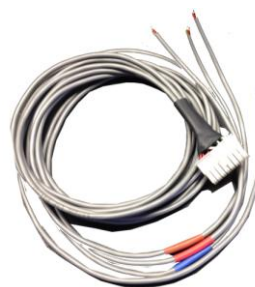
Cable Loom 2 (For Connector 2) This is sleeved in grey, each end is also colour coded with heatshrink
